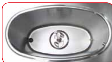
Elliptical tank in stainless steel and central stirrer
