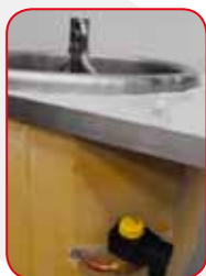
Half tank cooling control valve
